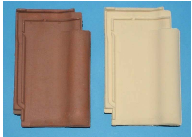
Figure 26: Crude red-brick ( \beta_s = 0.53 ) and painted one (light brown, \beta_s = 0.30 ).
