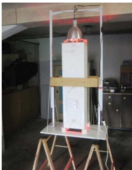
Figure 11: Heat radiation tube with an IR-spot [39].
