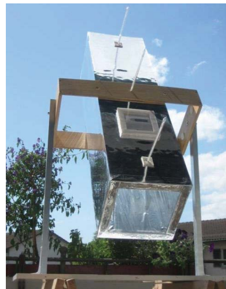
Figure 9: Optimized solar tube, adjustable towards the sun [39].
