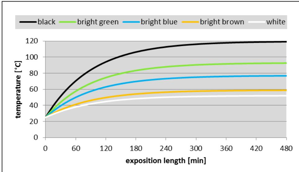
**Figure 5:** Temperature courses at differently coloured aluminium-plates
