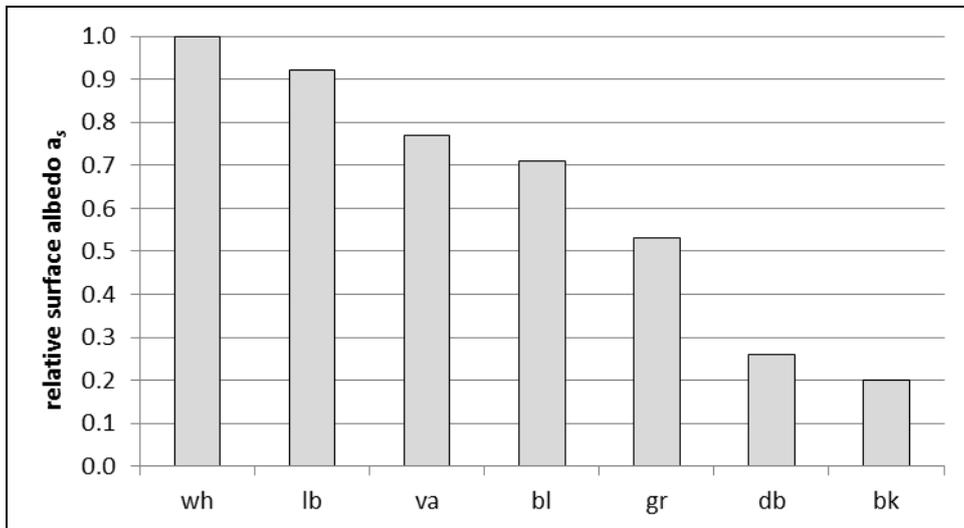
**Figure 9:** Relative surface albedos  $a_s$  on aluminium
