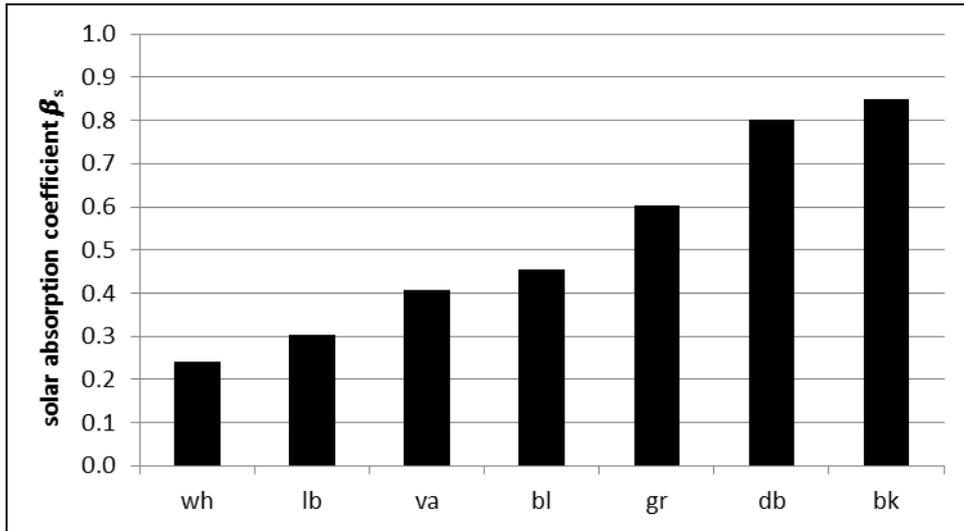
**Figure 8:** Solar absorption coefficients  $\beta_s$  on aluminium
