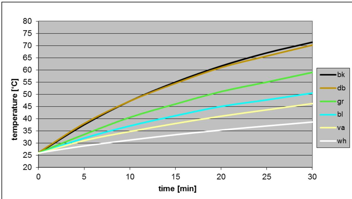
**Figure 4:** Warming-up of wood at  $970 \text{ Wm}^{-2}$  (method A).
