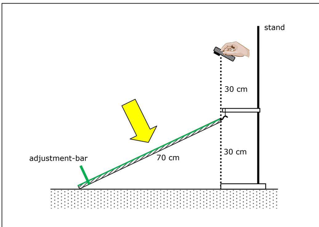
**Figure 2:** Assembly for the albedo-measurement by a light meter (method B)
