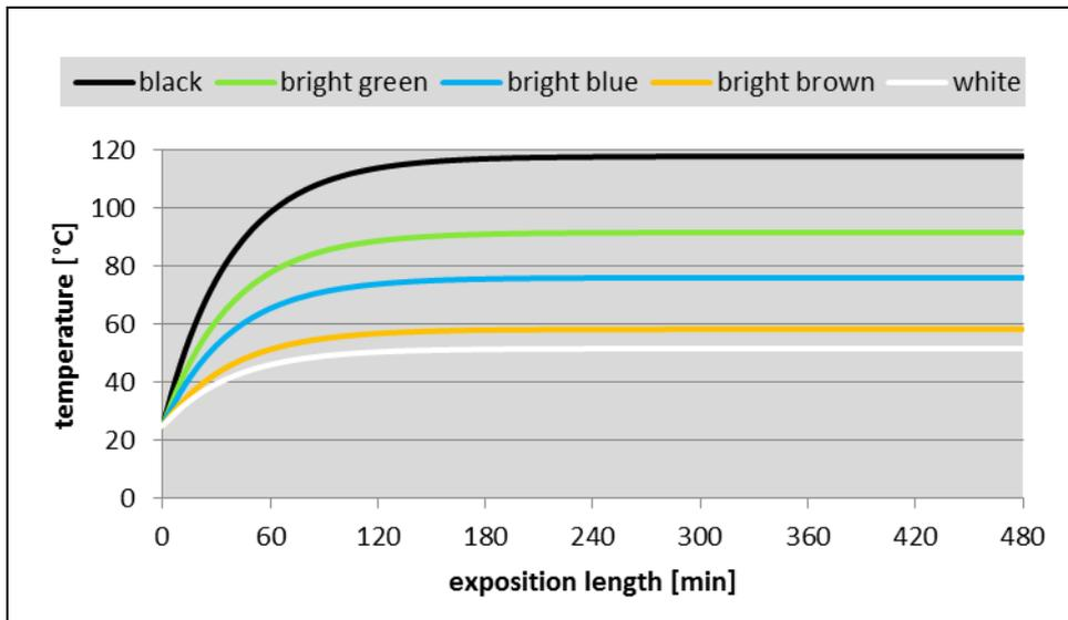
**Figure 6:** Temperature courses at differently coloured brick-plates
