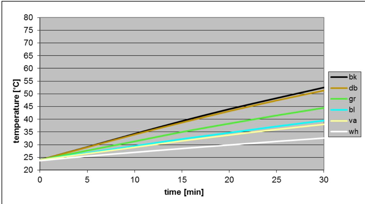
**Figure 3:** Warming-up of aluminium at  $1040 \text{ Wm}^{-2}$  (method A).
