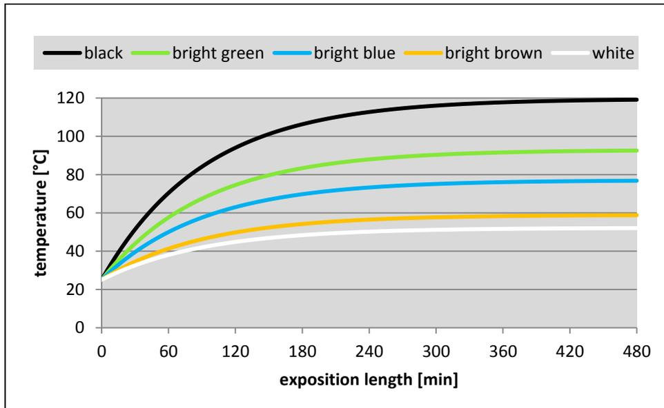
**Diagram 1:** Warming-up of aluminium-plates at a solar irradiation intensity of  $1000 \text{ Wm}^{-2}$  (plate-thickness 2 cm; with foil windows)
