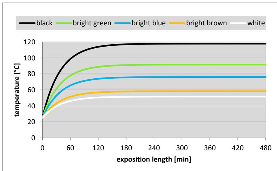
**Diagram 2:** Warming-up of aluminium-plates at a solar irradiation intensity of  $1000 \text{ Wm}^{-2}$  (plate-thickness 1,45 cm; with foil windows)
